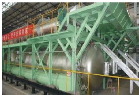
High-pressure impregnation tank.
